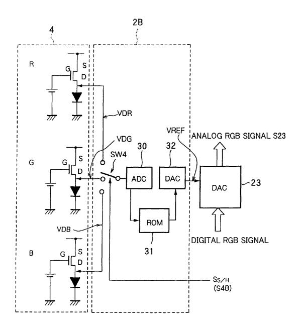
2B: LEVEL ADJUSTMENT CIRCUIT
