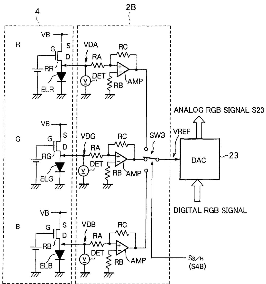
2B: LEVEL ADJUSTMENT CIRCUIT
