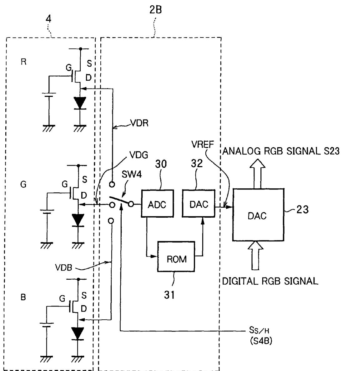
2B: LEVEL ADJUSTMENT CIRCUIT
