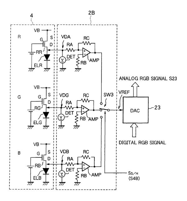
2B: LEVEL ADJUSTMENT CIRCUIT
